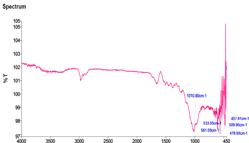
Fig. 10. IR spectra confirming the presence of organic acid functional groups during the Frankia consortium's e-fine particle leaching process.
