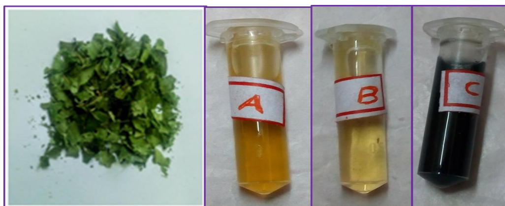
Fig.6.1 Color changes of iron nanoparticles fabrication a) FeCl 3 b) Green tea leaves extract c) After plant extract added with FeCl 3 solution
