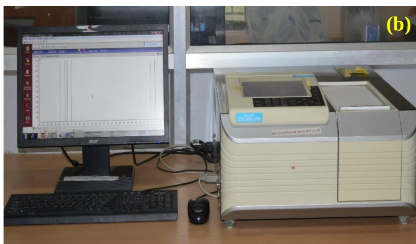
Fig. 2.7: (a) Schematic diagram of UV-Visible analysis (b) Photograph image of a UV2700 apparatus set up
