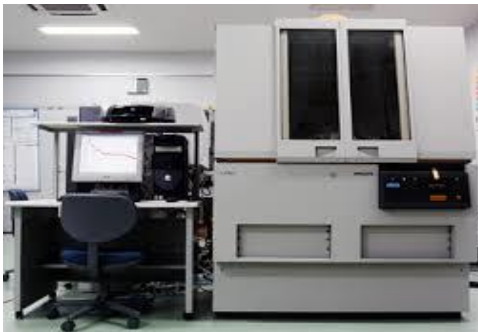
Fig. 3.10 Photograph of X-Pert Pro X-ray diffractometer
