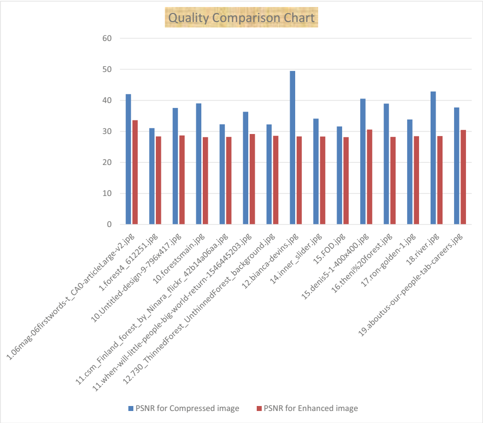
Fig. 5. The quality comparison chart for the raw image and compressed image based on its PSNR value.
