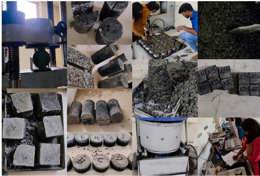
Fig. 7. Preparation of concrete and specimens.
