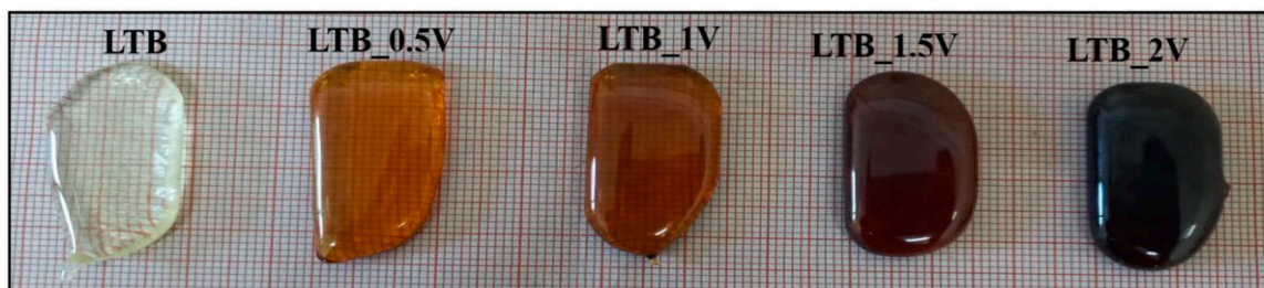
Fig. 1. Physical appearance of as-prepared LTB and vanadium doped LTB glasses.
