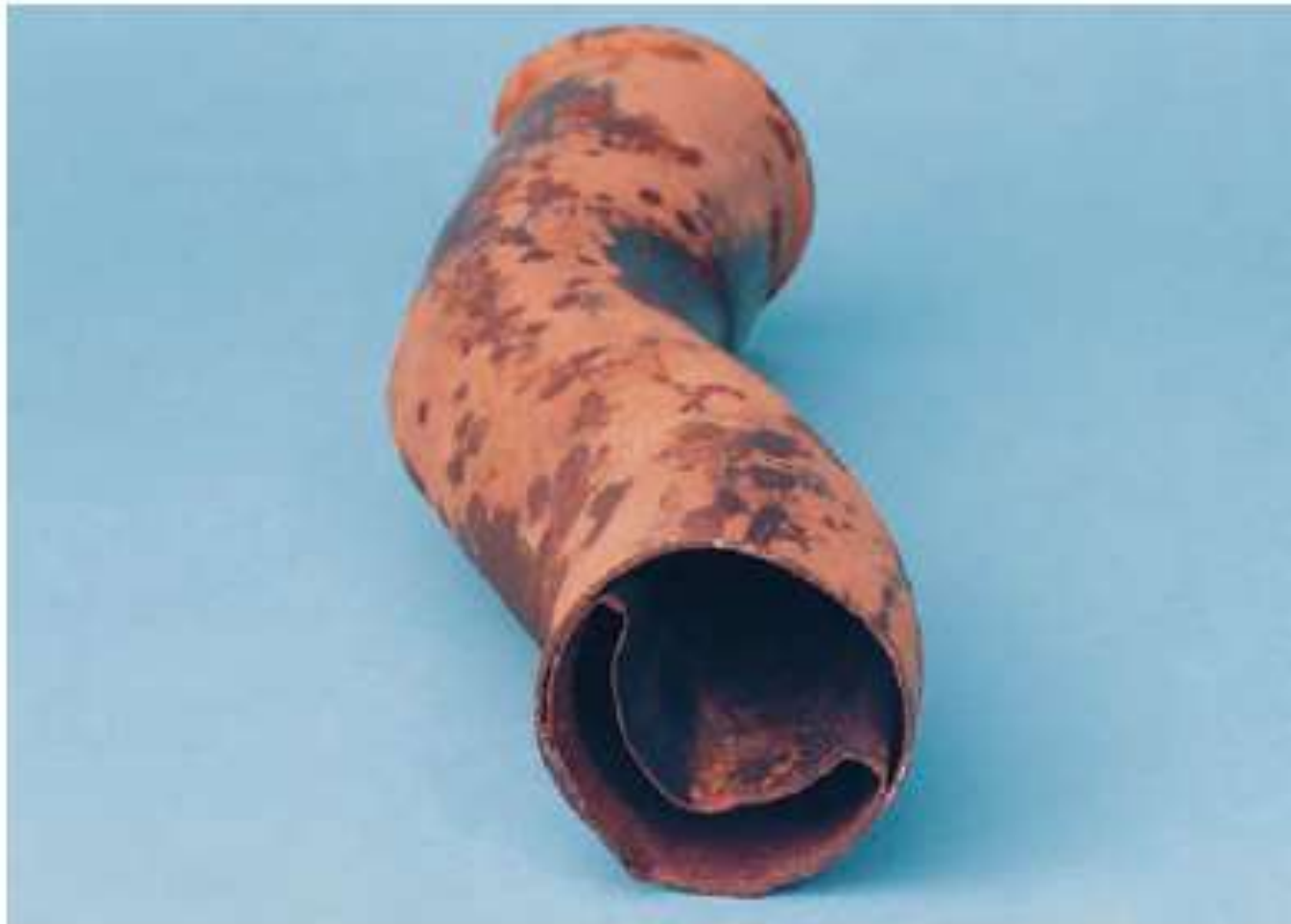
Figure 42.23 This collapsed laminated exhaust pipe caused breathing problems.
