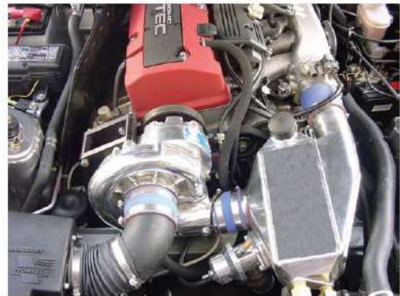
Figure 42.28 (a) A blow-through supercharger. (b) An aftermarket centrifugal belt-driven supercharger that is a fuel-injected blow-through design.
