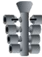
(b) Multiple patterns assembled to wax sprue
