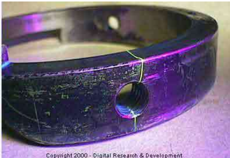
Magnetic particle wet fluorescent indication of a cracks at a fastener hole
