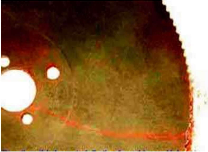
Indication of a crack in a saw blade
