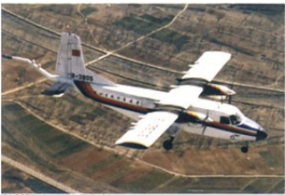
"Y-12" airplane installed with aeromagnetic system
