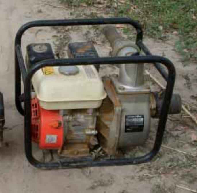
Motorized centrifugal pump
