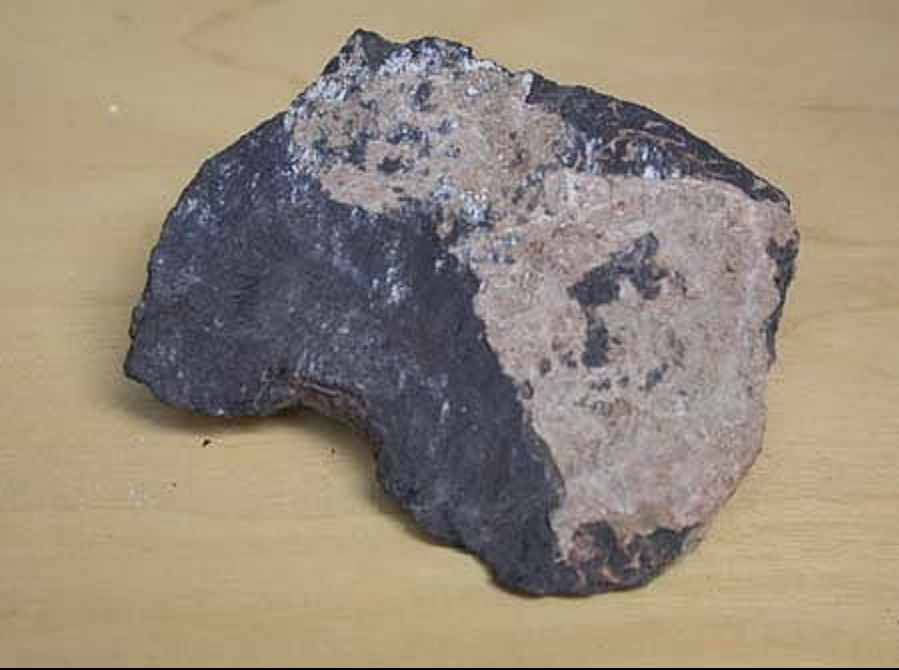
Massive black chromite in serpentine matrix Origin: Psonas, Euboea Island, Greece Sample size: 4.5 x 6.5 cm
