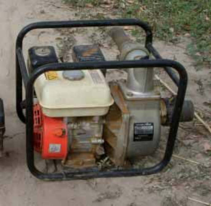
Motorized centrifugal pump
