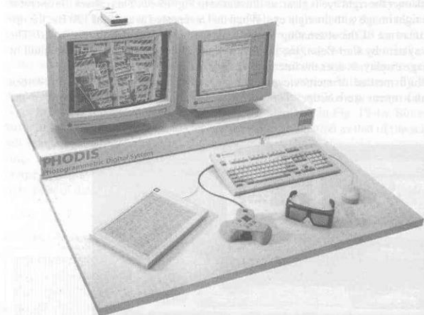
FIGURE 15-4 Zeiss PHODIS ST digital stereo workstation. (Courtesy Carl Zeiss, Inc.)
