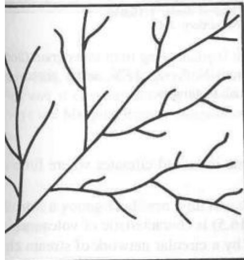
Figure 16.1. Dendritic drainage patterns: stereogram ( top ) drawing from stereogram ( bottom right ), and a classical drawing ( bottom left ). (From N. Keser, 1976, aerial photos from Geomatics and Mapping Branch, Government of British Columbia.)
