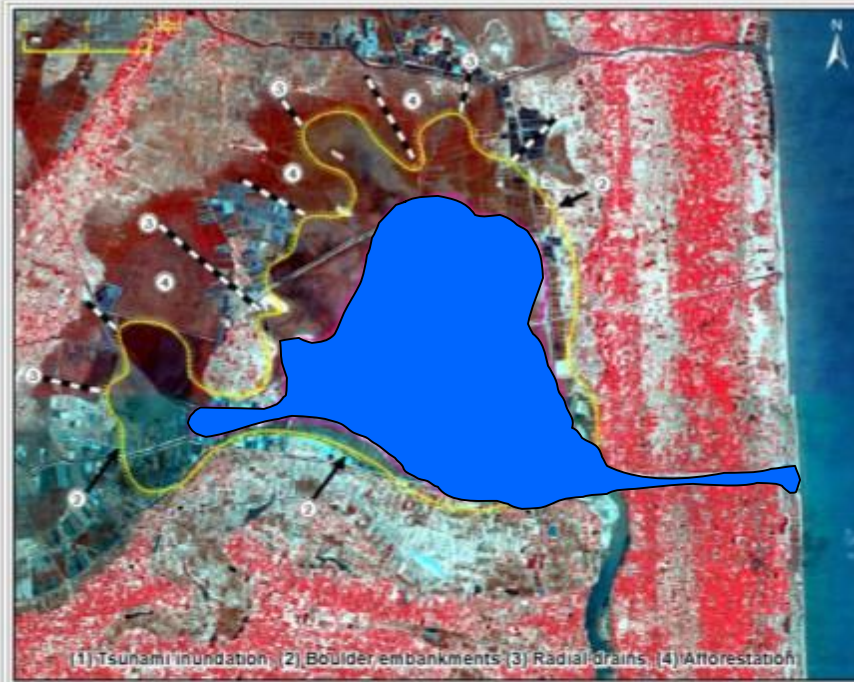
Fig.4.30 IRS P6 PAN merged image showing backwater - accommodators of tsunami surge
