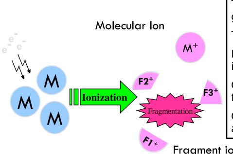
Thermal electrons emitted from filament hit gaseous molecules.
